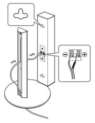
**3** Attach the speaker to the speaker stand with the supplied screws (large) securely after adjusting the height of the speaker.
